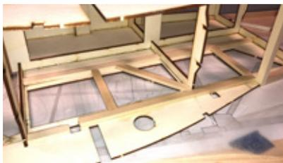
Glue all of these braces in position and hold them firmly in place while the glue cures. When cured, do the same for the starboard side of the fuse.
