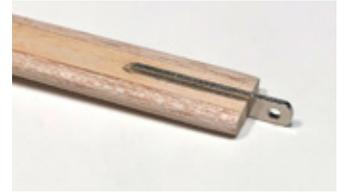
The slot should be roughly 1-1/4" long and the width of the metal strap's thickness. Now do the same thing for the other three blanks - but only on one end. Leave the other ends untouched for now.
