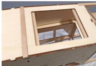
**Step 61 - Fuselage Assembly (attach H2 or H2A)**
