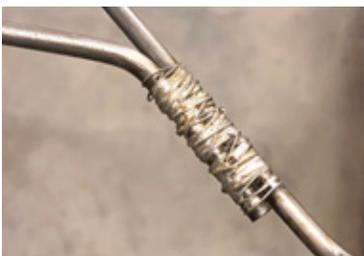
After cleaning, carefully and tightly wrap this joint with wire as shown here using. We used 26 gauge wire, but other thicknesses can be used.
