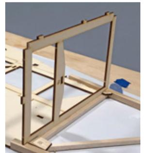
**Step 47 - Fuselage Assembly (TRAY, F5 and F6)**
