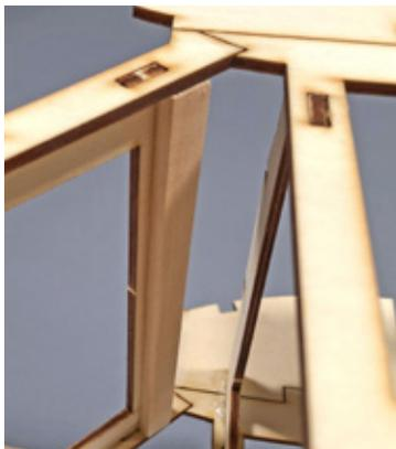
**Step 63 - Fuselage Assembly (F7 cross brace)**
