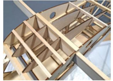
Now measure and cut the cross bracing that goes across the center section. There are three 1/4" square balsa pieces and two 3/8" square basswood pieces. Glue these in place as shown.
