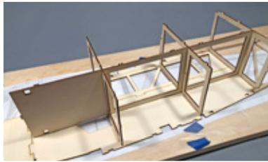
After satisfied with how this fits, remove it, apply glue and re-insert it to secure it in position.
