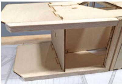
**Step 59 - Fuselage Assembly (attach P3, P4)**
