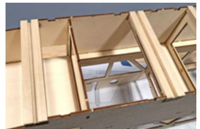
**Step 58 - Fuselage Assembly (fuselage corners)**
