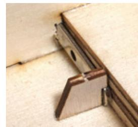
to one side than the other. The strap should be positioned so the end with the 2 closer holes is inside the fuselage, and the other end protruding from the fuse side by a 1/4" to 3/8". It also should rest flat against the 3/8" spruce cross brace.
