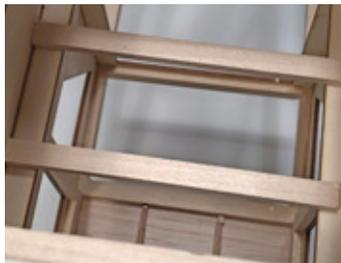
If using a glow or gas engine, measure and cut 2 more strips. These will be used for the throttle servo mount. Mount one strip on TRAY, just behind F5, then the other to span between the fuselage sides. It will need to be spaced for the width of your throttle servo. When satisfied with the fit and position, glue them in place.
