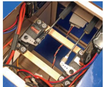
Finish the installation of your radio gear by adding the receiver, flight pack battery and the switch. We mounted the receiver to the fuselage side using a bit of self-adhesive hook-and-loop (not included).
