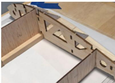
Fit as shown and make sure that the tabs completely slide into the slots in R8 as this will guarantee that R8 is held in vertically. When satisfied with the fit, glue R8 and WF4 to the bottom spar.
