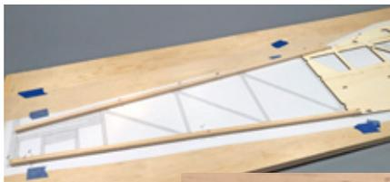
Note that the top longeron does not completely seat into the gap on top of the fuselage side. There needs to be a 3/8" gap for a cross support that is attached later.
