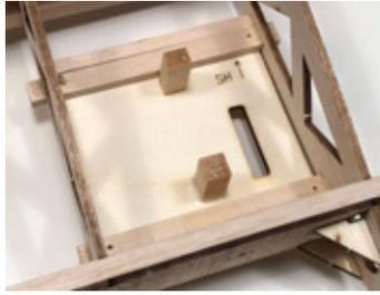
Now fit the servo hatches into position on the bottom of the wing. Using the pre-cut holes as a guide, drill four 1/16" mounting holes into the 3/16" x 3/8" basswood mounting strips installed earlier. Harden the wood with a bit of thin CA and you can use the supplied 2-56 x 3/4" self tapping screws to secure them in place.
