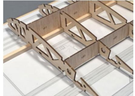
WB3 in place. When satisfied with the fit and location, glue these in place. Working your way inward, attach the other R7, WF3 and WB3 pieces in place.
