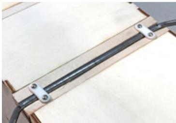
on the underside of the fuselage. Position the gear strut wires so they are centered on each LG, then mark and drill 1/16" holes where the straps should mount. Attach them using the supplied 2-56x3/4" self tapping screws.
