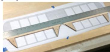
Again, it can make things easier to line up by using a long straight-edge as we've done in this photo.
