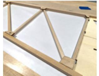
**Step 45 - Fuselage Assembly (fuselage starboard side)**
