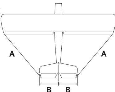
To be absolutely sure, insert the vertical fin down through the top fuselage slot, into the stab opening (this might require a bit of sanding on the fin for easy sliding). Once the fin is properly seated, measure the angle between the fin and stab. If at 90°, then it's correct. If not, reposition as needed.
