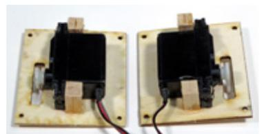
similar posts from the remaining pieces, sanding the ends flat. Position the aileron servo on the bottom of the aileron servo covers so the servo arm output shaft is centered in the opening.
