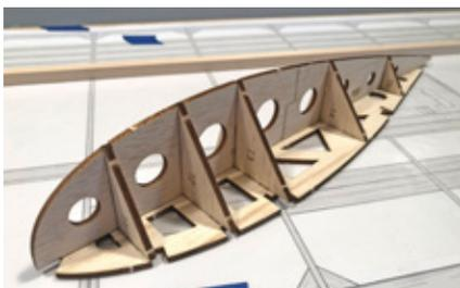
Then gently slide this sub-assembly into the notches in the R8A/B assembly from the last step. When satisfied with the fit, glue them together.
