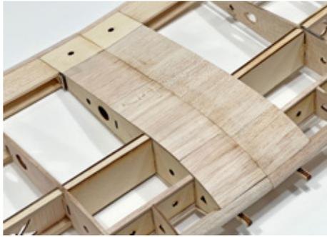
Remember, any twist in the alignment of the panels cannot be fixed after the epoxy cures and will lead to a poor flying model.
