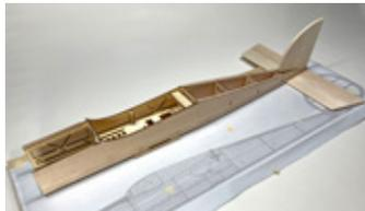
Sand as necessary for a good, slop-free fit. Then when satisfied, apply glue where the pieces touch and permanently attach the tail surfaces to the fuselage, as shown here.
