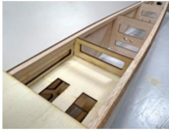
Make sure these are pushed completely into the notches of each former and glued to the outer sheeting.
