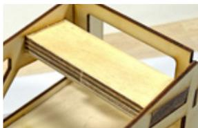
You'll now need to test-fit this into the large rectangle cutouts in the FS5 pieces. Sand as needed to get a good fit, then epoxy this into place as shown here. Clean off any excess epoxy with some denatured alcohol to keep things clean. Make sure that WH4 is perfectly centered as well.
