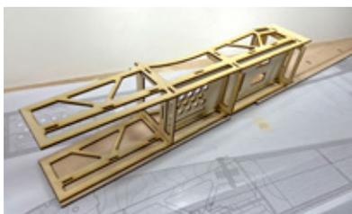
Now dry-fit the plywood box to the sheeting and note how it lines up. The left edges should align, and curved edges that make up the wing cradle should also be aligned. This will give a 1/4" gap along the bottom edge, which we'll take care of later.
