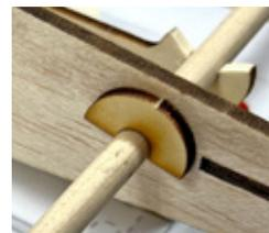
Wick thin C/A into any of these 1/2-circular pieces you use first, then snap them on to the dowel and use them as "stops" on each side of every rib. **WHEN YOU USE THESE, DO NOT GLUE THEM IN PLACE** - they are meant to be removable - and re-positionable.
