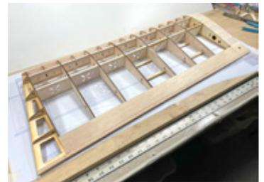
*Set the port wing panel aside and begin work on the starboard wing panel. Tape the starboard wing plan and fresh wax paper on your board. Then follow steps 80 through 115 to complete the starboard wing half. Once finished, then move on to step 116.*
