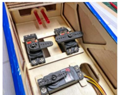
When mounting the rudder and elevator (and throttle, if glow) servos, we've included TR4s (LP1) to double-up the ply where the elevator and rudder servo's
