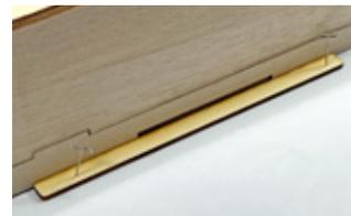
In the photo you'll see a long punch-out of lite-ply from the FS5 pieces (you should have two). These make great "tools" for holding the fuselage in place over the plans during the next couple of steps.
