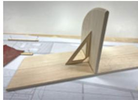
It's time to glue the fin to the stab. Place the stab so the hardwood tailwheel mount is against the board (not-seen).
