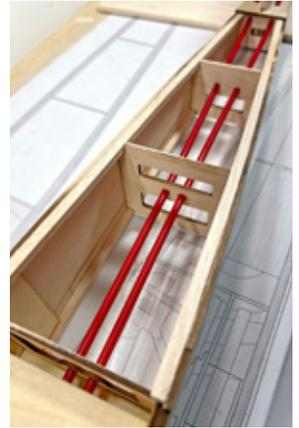
You'll note that there are small pre-cut circles in each of the F5, F6, and F7 formers, as well as cutouts in FS6, on each side of the vertical fin. These are the areas where you will slide the outer tubing through. Make sure you glue them to each of the formers so they won't move and/or rotate over time.
