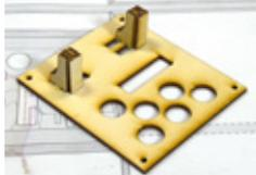
When finished you should have a complete aileron hatch, that looks something like this third photo, just without the covering. Now using the other SH1 and SH2s, make the other aileron hatch - again making sure it's mirrored from the first one.
