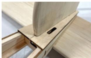
Now CAREFULLY test fit this around the vertical fin, so it lays against the fuselage and stringers you just installed. Sand as necessary for
