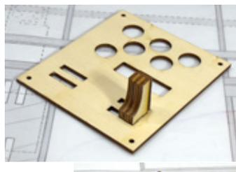
Now remove the servo and the SH2s, apply glue to the base of the SH2s and attach them to SH2, similar to what's shown here.
