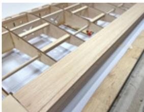
Glue the rear sheeting in place on the rear of each rib overlapping R2A, all the way out to R6, making sure it slips into the groove cut into each rib. It should be flat along its entire length and also glued against the trailing edge strip.
