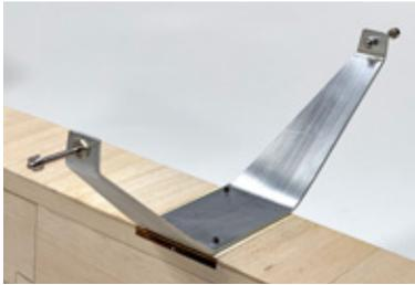
Center the main gear on the LG1 block you mounted in the bottom of the fuselage. Make sure it's aligned straight and true. Then mark the 4 mounting holes and drill these four holes through LG1 with a 1/8" drill bit. Attach the gear to the fuselage with the four hex-bolts, securing them on the inside with the four t-nuts.
