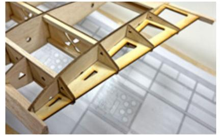
When smooth, locate T1 from LP2, and one T2, T3, T4, and T5 from BP2. Check the plans to see the order that T2-T5 fit on to T1.
