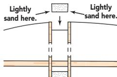
Gluing this in the piece this correctly will take a bit of time, so we recommend against using an instant setting glue. If you are using CA, use a thicker formulation that gives you a bit of working time.
