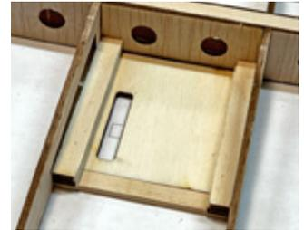
When satisfied with how these are installed, carefully glue them in place to the ribs, the web and where it touches SW3. But DO NOT GLUE THEM TO SW1.
