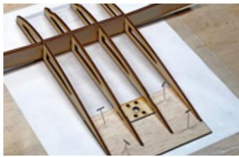
Make sure the ribs are straight and true and glue them in position, making they're pressed flat against the building surface.
