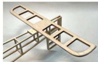
When you have it in the correct spot, use a pencil to draw some alignment marks onto the stab, where it intersects the fuselage. Then remove the stab, apply some glue and attach it permanently right back in the place it was.
