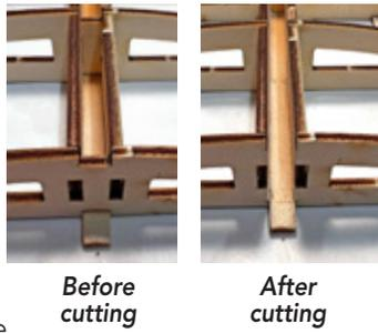
After cutting, make sure that the area is completely clean and smooth, as this will form 3 sides of a box where the dihedral brace will slide through. The cleaner/smoothier it is now, the easier it will be to slide in the brace when it's time.
