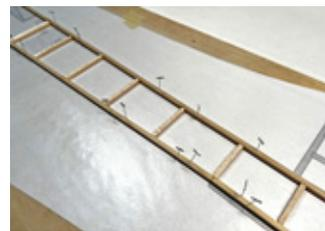
Carefully measure, cut and bevel each piece for a nice, proper fit and glue each in position as you go along. They should all be nice, straight and flush with the longerons. Take your time and make it something you can be proud of. *Remember, that most of this will visible when the Minuette is completed, so make it count!*
