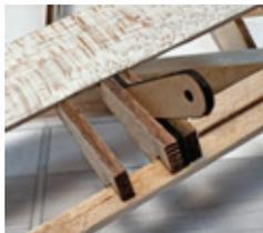
Now before I start this step, I'm gonna put this out there for your consideration. What you'll form with these three pieces is the control horn of the aileron. Horn itself is made from 3-ply plywood and will be reinforced by wicking thin CA into it.
