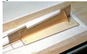
Now you'll attach the left fuselage framing to FB. Working and gluing a little bit at a time, make that the framing runs true along the length of FB.
