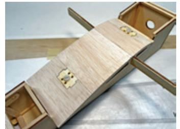
Use caution to make sure the wing does not move until both holes are drilled.
