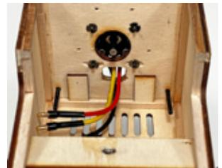
You'll also need to make a hole underneath the motor to allow the motor's wires to pass through the firewall, into the fuselage.
