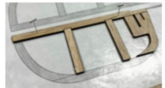
**Step 57 - Horizontal Stab Assembly (ST9)**
