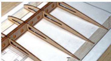
as you've used before. Then install another pair of SW3s, R4, two more SW3s, then R5. And finally you'll install the remaining pair of SW3s and the R4.
