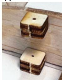
Also note that the WAs that attach to the rear end of R5 are offset slightly to allow them to fit within the wing's thickness.
