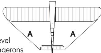
The distance from the port stab tip to the port wing tip should be the same as the starboard stab tip to starboard wing tip.
