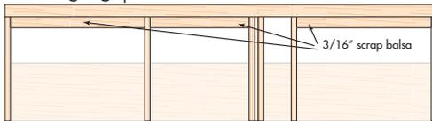
**Step 30 - Wing Assembly (Anchor supports)**
