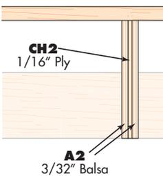
Once the glue has cured, you can remove the aileron from your building board and attach CH2. Note that the long horn on CH2 should protrude out the bottom of the aileron. Glue this in place up against the A2 you just installed. Now glue the remaining A2 in place, up against CH2. Lastly, using a bit of thin CA, wick it in all around the end of CH2. This will strengthen it even further.
