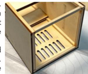
One will go across the bottom, glued to the sheeting and side framing. The other will spanning the distance between top of the fuselage sides.
