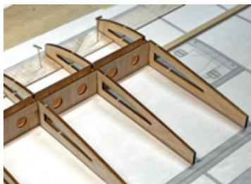
satisfied with how these pieces fit, glue them in place, making sure they're aligned and all tabs are properly seated. The bottom edges of the SW3s should be glued to the sides of the lower spar and the rib should be flat against the plans.
