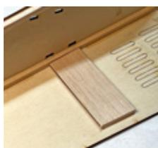
Then glue LG1 on top of the LG2s, making sure it's aligned properly when by fully inserting both tabs into the pre-cut holes on the fuselage side.
