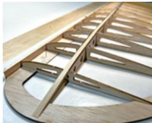
To install this piece, first lightly sand the edges of the bottom face of the spar as shown in the drawing to the right. This will help the spar slide in easier.
