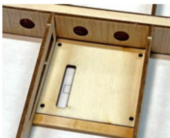
place on the plans, between the ribs and up against the lower spar. Now SW3 will be installed to form the 4th side of the aileron box. It should be snug up against both ribs, and loosely against SH1. I say loosely because you'll want to leave a touch of room to account for the thickness of covering to be applied later.
