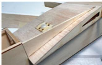
Looking down from the top, use a pencil and straight-edge to lightly draw a line onto the wing's center section sheeting, denoting a continuation of the fuselage's outer edge.
