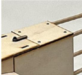
Then use four 2-56x3/4" self tapping screws to hold on each of the hatches.
