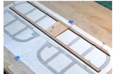
**Step 52 - Horizontal Stab Assembly (ST3)**
