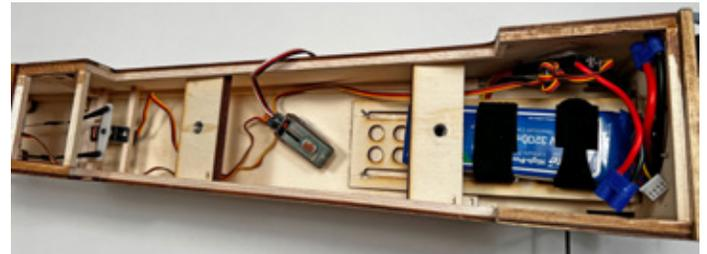
Finish the layout of your radio gear by adding the receiver, flight pack battery, ESC, and the switch (if using one). We mounted the receiver to the tray by using a bit of self-adhesive hook-and-loop (not included). The ESC was mounted to the inside wall of the fuselage in the battery area.
