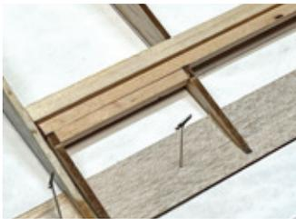
Cut one piece to fit into the outer gaps on each end. Then the other one should fit into the large gap in the middle of the aileron, as shown in this diagram, and on the plans.
