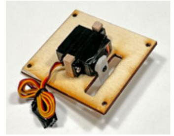
Position your aileron servo on the inside of the aileron hatch so the servo arm output shaft is centered in the opening.
