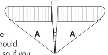
When finished, center the wing's center section into the saddle. Now align the wing properly to the fuselage by adjusting as needed so that distance from the port wing tip to the rear of the fuselage is the same the distance when measured from the starboard wing tip to rear of the fuselage.
