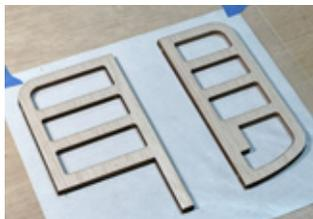
When the glue has cured, remove these assemblies and flip them over and lightly sand the framework. Then glue the other set of VF12/VF13 to the assemblies.
