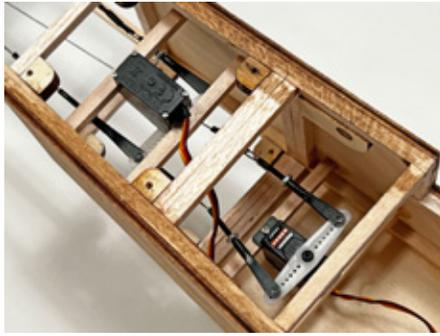
These photos shown examples of servo installation in one of the Minuette prototypes. As you can see, we've used Dubro's 2-56 pull-pull setup for the elevator and rudder and it works very well. You can use other systems, but a pull-pull system will look best as it's more "period correct".
