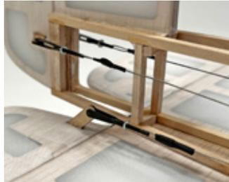
We used some of the leftover 3/16" sq. basswood to form the servo mounting beams inside the fuselage.
