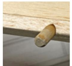
Place glue on the lower part of the dowel and insert the dowel through the leading edge and into WH1, leaving approximately 1/3"-1/2" of the dowel exposed.
