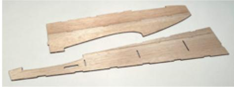
Glue one FS1 to one FS2, making sure that all the tabs on FS1 are completely seated into the notches cut into FS2. Also make sure that the pieces are flat along this entire joint.
