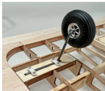
landing gear straps as shown in the photo. Use a 1/16" drill to make the mounting holes for the screws, and then attach the straps in position.
