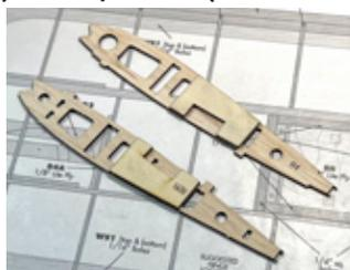
(towards the wing root). When glued in place, R2A and R4A need to be perfectly aligned with top and bottom edges of their respective ribs. Also the rear edge should be just on the edges of R2A and R4A should be aligned with the rear spar cutouts in each rib.
