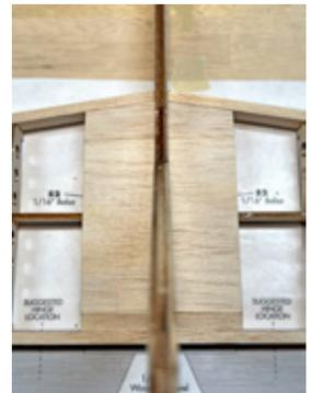
Using the same techniques that you used when forming the wing's center sheeting, measure and cut 3 total pieces to make each sheet. Take your time when measuring and cutting - especially against the tapered edge of the leading edge. What you want is a piece that fit snugly against the leading and trailing edges as shown here.
