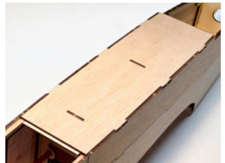
When satisfied on how this fits, remove, apply glue and then attach in place.
