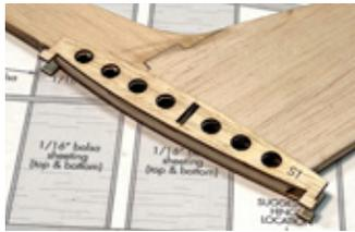
Make sure these are properly aligned, and straight with each other. Refer to the drawing of this section shown on the side view of the fuselage plans.
