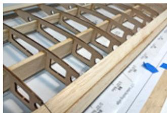
As the sheeting we get can vary in density, you might have to apply a bit of Windex® glass cleaner to loosen up the grain and allow it to bend without cracking. Soak the outer side of the wood to expand the fibers. Now hold it to curvature needed, then use a hair dryer or covering heat-gun to help "set" the balsa's bend as it dries. Once dry, then you can glue it in position.
