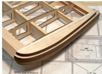
**Step 36 - Wing Assembly (aileron box)**
