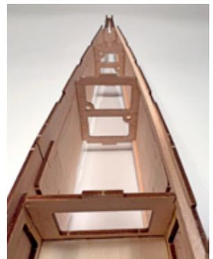
*You'll need to remove any pins/tape holding the rear of the fuselage together for the next few steps.*
