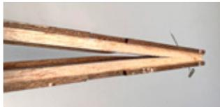
Using a ruler and straight-edge, measure and draw sanding-guides starting at the rear of the top and bottom stringers, tapering in about 1-1/2". These marks will show roughly how much wood should be sanded away on the insides of each fuselage side, so they will taper correctly. Although you can cut this with a saw or hobby knife, sandpaper makes quick work of this, but use caution not to remove too much.
