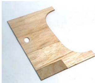
It's easier to join the shorter lengths of sheeting together on a flat surface. Then when the glue has cured, glue the sheeting in place on the wing. Start at the leading edge and gluing a little at a time. Press the sheeting firmly against the ribs and wait for the glue to cure before gluing the next section of sheeting - slowly working your way back to the trailing edge, being careful not to put a bend (warp) in the wing.
