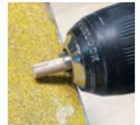
Now mark and cut a hole into the leading edge of the wing where the dowel should be inserted, making sure it is centered on the leading edge strip. Cut the hole a bit undersized, then gradually enlarge it until you get a nice, snug fit. Test fit the dowel and make sure that it also slips through the internal WH1 piece.
