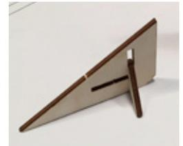
We recommend using this triangle throughout the wing construction, and in the alignment of the vertical fin.
