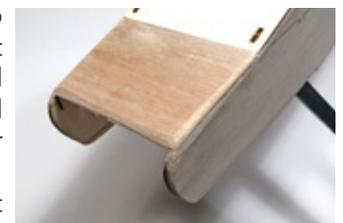
you also sheet the area on the top of the fuselage, between the front sides, as shown here. This not only adds to the looks of the Javelin, but gives much needed support to the sides so they can handle vibration and airflow much better. If using glow lower, you will need to make cutouts for the needle valve and muffler screws.
