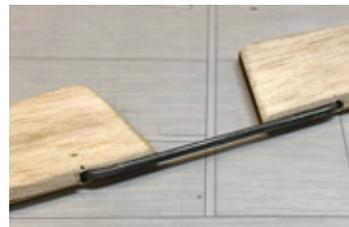
Temporarily tape the elevator halves in position on the stab.
