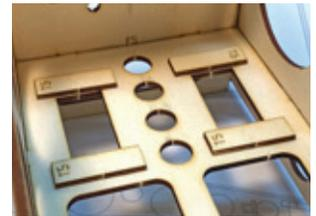
Locate four T5s from LP3, LP4 and LP6. These are glued in place as shown to double-up and strengthen T2, where the mounting screws will be threaded in.
