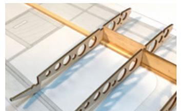
Now, glue R5 in place. When it is properly aligned, the SW1 tabs will be fully seated and R5 will be at a 90° angle to the building surface. Also tack the rear tab to the waxed paper.
