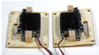
Note that the left hatch is a mirror image of the right hatch. Now fit the servo hatches into position on the bottom of the wing. Using the pre-cut holes as a guide, drill four 1/16" mounting holes into the 3/16" x 3/8" basswood mounting strips installed earlier. Harden the wood with a bit of thin CA and you can use the supplied 2-56 x 3/4" self tapping screws to secure the hatches in place.
