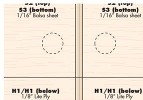
This is optional, but could make the aileron servo installation a bit easier, once the wings are covered. Cut two 18" lengths of string, one for the port side, and one for starboard. Starting with the port wing panel, push the thread through this hole, then through the circular holes in R3, R4, R5 and R6. The string will now extend from the servo bay, out through the bottom of the wing. Tape both ends of the string so they won't easily pull out. Do the same for the starboard side.
