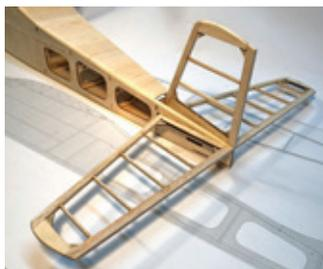
Mark and trim the 1/4" framing so it will allow the rudder to clear.
