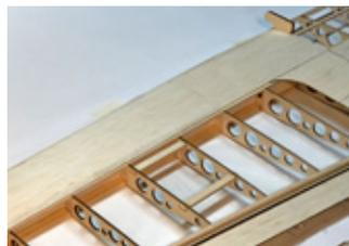
It's best to glue the forward edge of the sheeting to the leading edge first. When the glue has cured, apply glue to the ribs, then gently wrap the sheeting around the curvature of the wing ribs.
