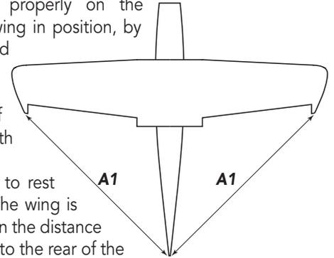
Then allow the wing to rest in the wing saddle. The wing is perfectly aligned when the distance from the left wing tip to the rear of the fuselage is the same the distance when measured from the right wing tip.
