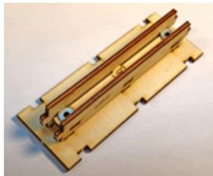
When assembled, then push this assembly into the slots cut into the middle of WB8. Make sure these are all fully seated, perpendicular to each other and firmly glued in place.
