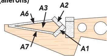
Notice the tab extensions. They all have a unique cutout where A1 lays at a 45° angle. Locate both A1s and lay them into the slot as shown here, centered side to side along the space for the aileron (do not glue).
