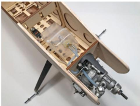
mounting it as shown here on one of our Javelin prototypes. This particular engine required a muffler extension to space the muffler away from interfering with the bottom of the fuselage. Holes will also need be drilled for the throttle pushrod to pass through into the fuselage.
