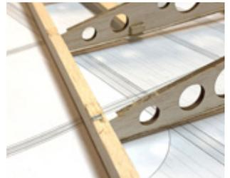
But the tabs on R4-R9 will also need to be trimmed 1/16" below the trailing edge. This will allow the cap strips to be flush when installed.
