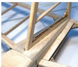
Once glued in place, sand these pieces to blend into the fuselage.
