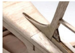
Make sure it is straight when attaching. Then sand to blend into the vertical fin.
