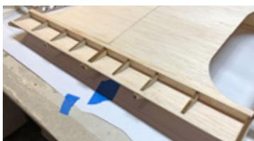
the sheeting, in-line with the R4 ribs to form the caps of this rear section. Then glue two more A4s half way between the R1A and A4s.
