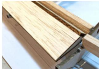
When satisfied, glue A6 in position, making sure it is glued to the rear or A7, all of the A3s and to A2.
