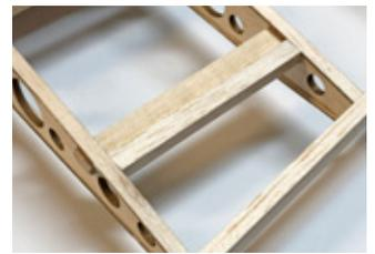
This is not a structural piece. Instead it is a trim piece that aids in covering later on, as you'll have to cut out the covering in this area to install the servo and hatch.
