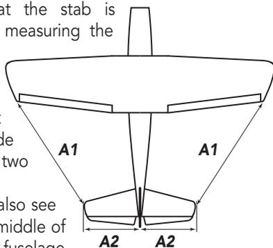
When aligned, you should also see that the pre-cut slot in the middle of the stab is centered in the fuselage.
