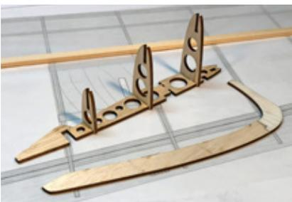
TP5 into their respective notches in R10. Make sure each of these pieces are glued in at a 90° angle to the R10, and pay attention to the orientation of these pieces as it is possible to insert them the wrong way. The small etched circles are to be oriented to the top of the wing (the edge with the tab on it).
