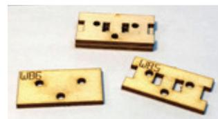
When gluing them together make sure the holes are aligned between the two pieces and that the outer edges are also aligned.
