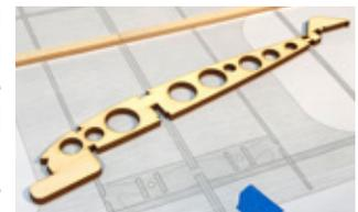
spars, sub-spars and other pieces in the following steps. Hold this assembly flat by weighing it down on a flat surface as it cures. Once cured, wick thin CA generously into the lower wing tab to help strengthen the wood.
