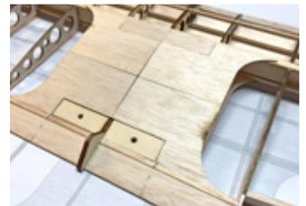
Glue these in place as shown, using the same technique used when attaching the bottom center sheeting.
