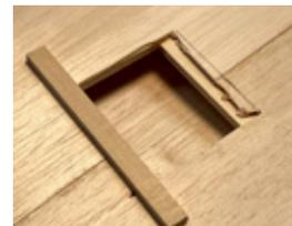
Then carefully cut away the fore and aft edges of the box so the sheeting is flush with the lower spar and the rear frame of the aileron box.
