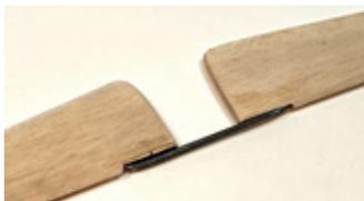
Now place the elevator joiner on top of the elevator halves and mark where holes will need to be drilled.
