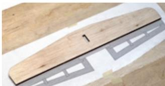
When the glue has cured, remove these assemblies and flip them over and lightly sand the framework to prep for the lower sheeting.
