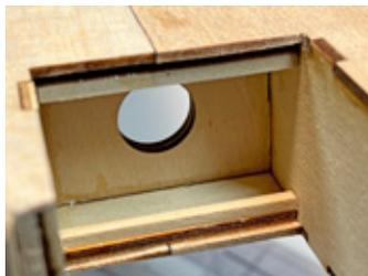
Also locate the 3/16" x 12" sq. basswood strip. Cut two 2-1/4" lengths, then glue them to the edge of the FES pieces you just installed. These two pieces will give more surface area for the electric firewall to grab on to, in the next step.
