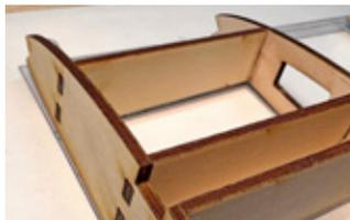
here. When R1 is properly installed (with the tabs in SW1 and SW1B fully inserted and TE inserted on the trailing edge), it should be perfectly flat and the same 5° angle along its entire length.
