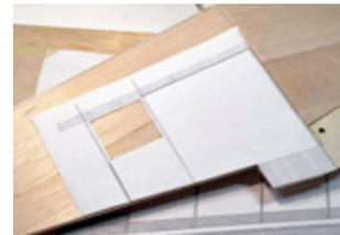
The rectangular cutout is pretty close to the size, but I advise lightly cutting inside it by 1/8" or so - using just enough pressure to cut through the outer sheeting. You should now have a hole that reveals the hatch rails, similar to what's shown here (except hopefully a bit neater than my example).
