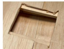
An easy way to find the sides of the box is to take a piece of scrap 3/16" x 3/8" and place it directly over one of the servo rails, mark, then cut this outer edge. Do the same to find the outer edge of the other rail.
