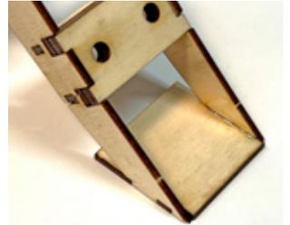
Glue in place as shown, again making sure all its tabs are fully seated into the slots of both SC4s.
