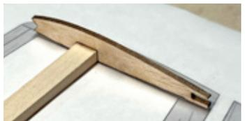
I like to put a small drop of medium CA on the bottom of the backside tabs of each rib to help lock it in place to the waxed paper (or you can use pins if that's your thing). Also make sure to use the included triangles that you should have at hand from the first step of this build. Using the triangles ensure that this rib, and all subsequent ribs are perfectly aligned at 90° to the building surface.
