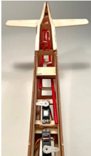
Also when installing the outer sheath of these sorts of pushrods, you'll need to tack them to the fuselage structure in several places so they won't move or bend while in action.
