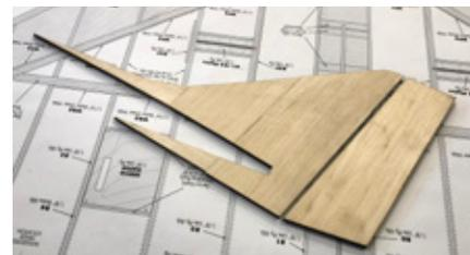
The piece shown separated from the fin is the rudder (VF5). We have flown the Comet with and without rudder and you can choose
