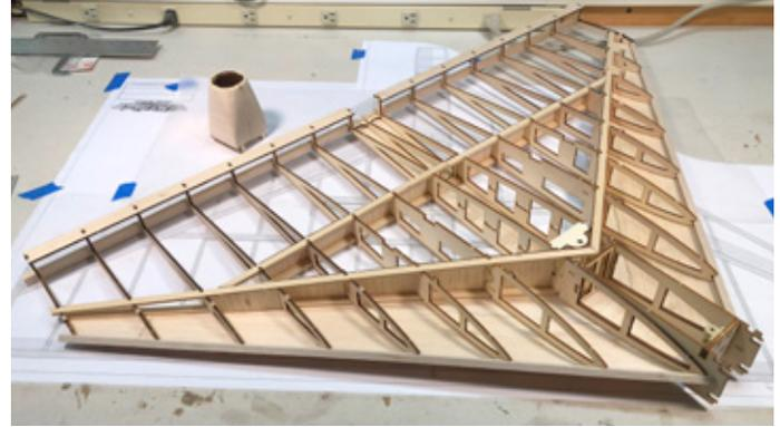
Once all the glue has cured, remove the Comet assembly from the building surface and flip it over.
