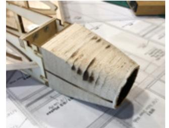
Now, to hold the cowl in position, drill into the holes in each cowl mounting tab using a 1/16" bit. Make the holes about a 1/2" deep. Using 4 of the supplied 2-56 x 3/4" self tapping screws, attach the cowl to the Comet.
