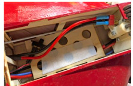
For electric power, locate TF from LP3. This can be glued in place and used as the "floor" to mount the flight battery to using a bit of hook-and-loop (not included).
